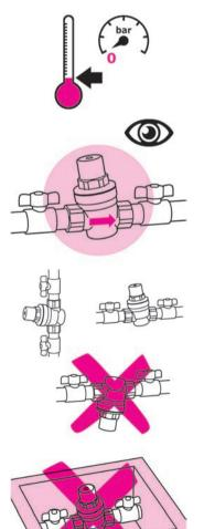
Assembly and disassembly should always be carried out while the system is cold and not under pressure.
