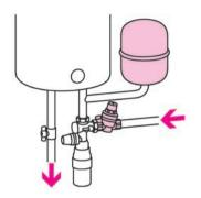
Install an expansion vessel (between the pressure reducing valve and the water heater) to absorb the pressure increase downstream of the reducing valve (when this is closed), caused by the water heater exceeding the specified temperature.
