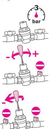
The 5334...H and 5337...H series reducing valves are factory set to 3 bar
