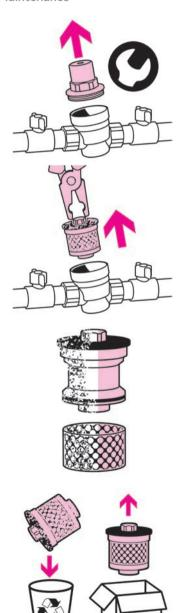
It is recommended to carry out maintenance and cleaning of the removable cartridge on a regular basis and if the reducing valve does not maintain the set value.
